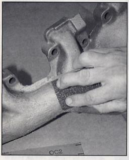
After the putty has air dried, smooth it out with a file and 80-grit sandpaper. This will be the hardest part of the repair because the putty dries rock hard. You do not want the Pyro-Putty to be perfectly smooth over the crack; the cast-iron exhaust manifold has a rough surface, so if you make the repair perfectly smooth, it will be noticeable.
