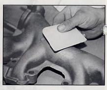
Use the Bondo spreader to evenly work out the compound and then feather the edges. Spread the compound a little higher than the crack to allow for the slight shrinkage that will occur. Let the compound air dry for five to seven hours at room temperature.
