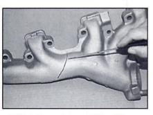
This is the crack in our Fairlane GT ex-🚄 haust manifold that we will repair. Do not try to fill cracks exceeding 3/8-inch wide.
