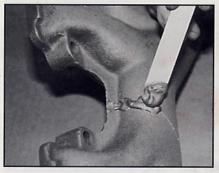
Thoroughly mix the Pyro-Putty metal repair compound. Using the wooden spatula provided, spread it down into and on the crack. Make sure it covers completely. If the putty does not smooth out, add about one tablespoon of thinner.
