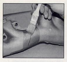
4 After you have finished sandblasting, clean all of the sand and residue from the manifold. Thoroughly clean the crack with lacquer thinner.
