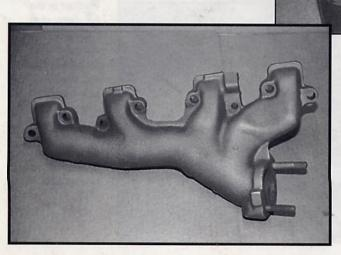
After the manifold has dried to the touch, you can reinstall it. Start the engine and let it run for approximately 10 minutes and the Pyro-Putty will be totally cured to full strength. The manifold is not only repaired, it also looks like new. Just like magic. MCR
